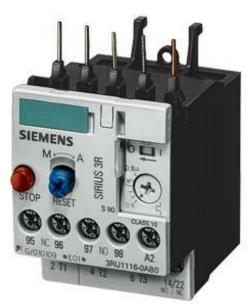
Overload relay 7...10 A For motor protection Size S00, Class 10 Contactor mounting Main circuit: screw terminal Auxiliary circuit: screw terminal Manual-Automatic-Reset !!! Phased-out product !!! Successor is SIRIUS 3RU2 Preferred successor type is >>3RU2116-1JB0<<
